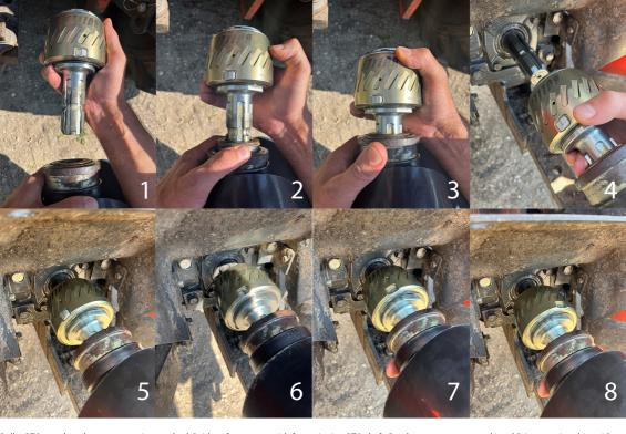
Bullet PTO coupler adapter connection method Guide - for tractors with free spinning PTO shaft. Read your owners manual in addition to using this guide.
