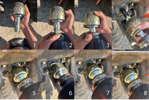
Bullet PTO coupler adapter connection method Guide - for tractors with non free spinning PTO shaft/ PTO brake. Read your owners manual in addition to using this guide.
